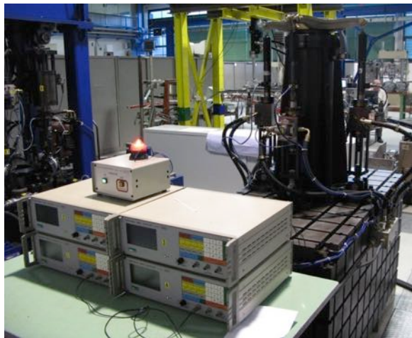
AW 109 Swashplate Rotating Assy Fatigue Test
