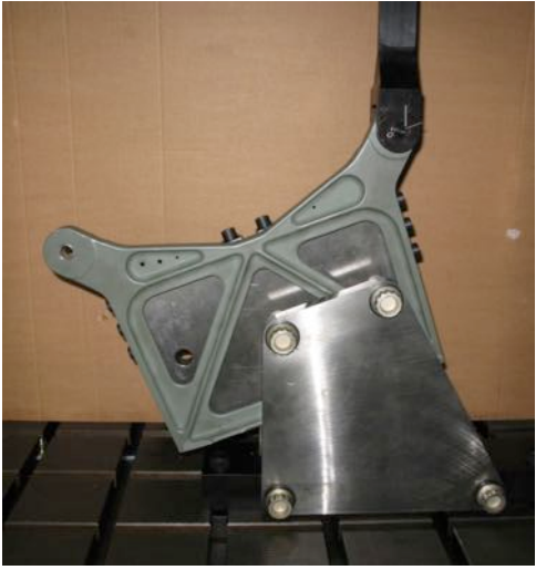
Sea King Tail pylon fold joint upper hinge fitting fatigue test
