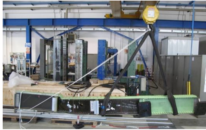
NH 90 Input case Fatigue test
