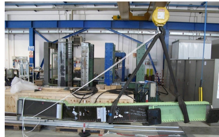
NH 90 Input case Fatigue test
