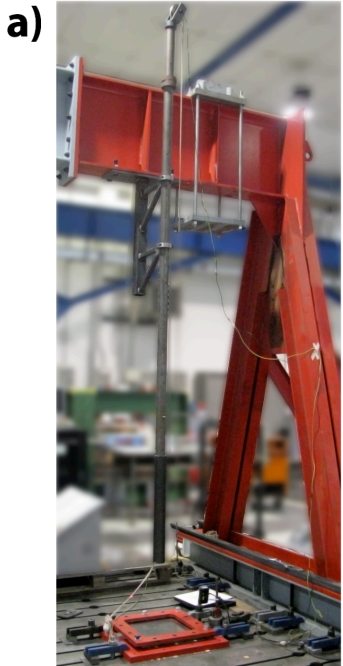
1) (a) test rig for the drop test; (b) focus on the rigid frame for panel grounding and (c) examples of sandwich panel specimens after impact tests.
